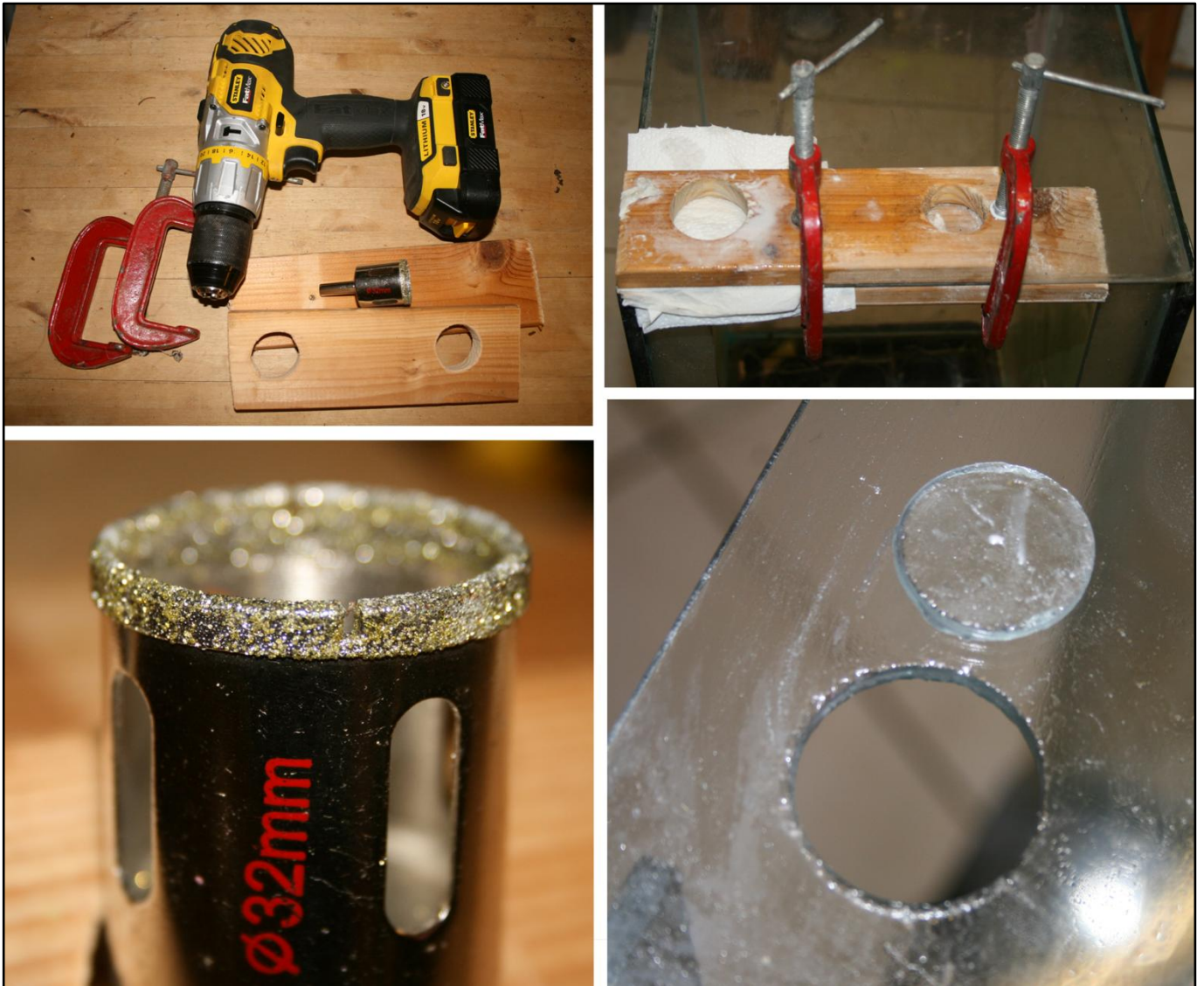
Equipment and technique for drilling holes in glass aquaria. A standard drill/driver, C-clamps, a diamond-coated glass hole cutter, and plywood jigs to prevent wandering of the cutter. Breakage and cracking of glass adjacent to hole is minimised by bracing with plywood. It is important to drill at low speeds and with plenty of water to help cool the cutter and glass during cutting. Photos: M. Walters.
