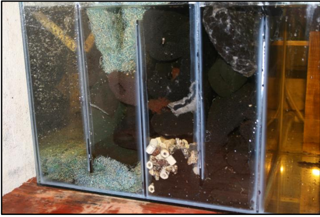
Sump with filter media installed and filled with system water. Photo: M. Walters.
