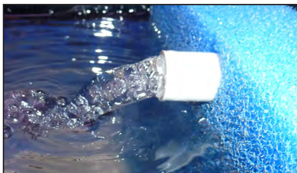
Tubular formation of the bubbles efficiently moving the maximum amount of water.
