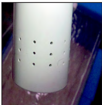
The lifter tube end with the air slieve removed.
